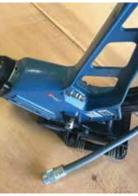
Your air hose should have a minimum of 150 psi (10.6 kg/cm2) working pressure rating and be fitted with a quick-disconnect fitting at the tool.
