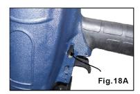
Original factory setting is single sequential trigger mode.
